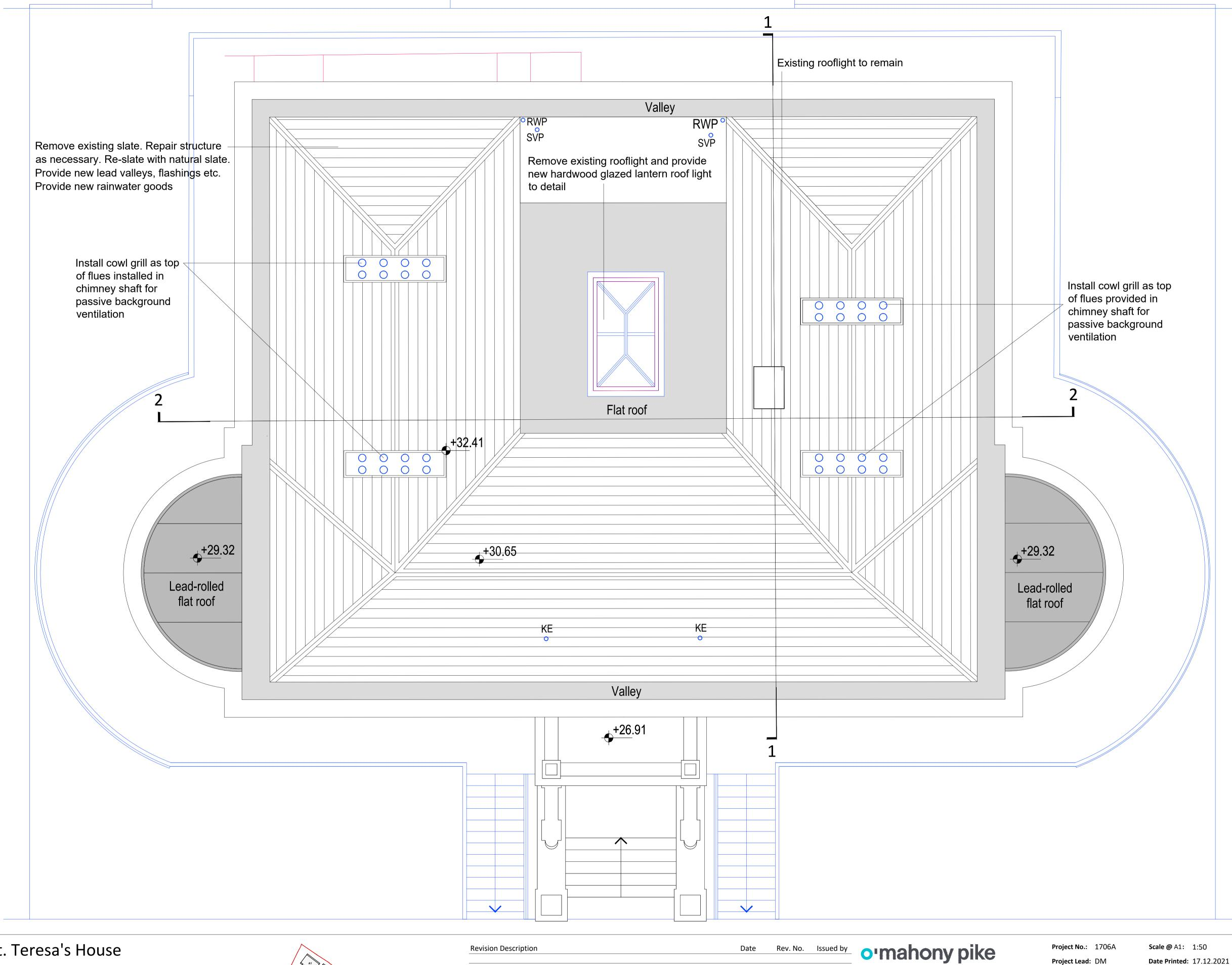
KE - kitchen extract RWP - rain water pipe SVP - soil vent pipe
